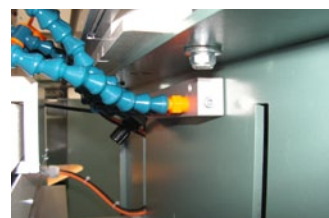
The pad air diffuser device can also be mounted magnetically .
