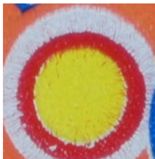
Example of a poor print caused by electrostatic charge
