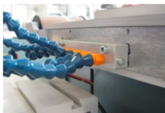
The pad air diffuser device can be mounted with screws horizontally .
