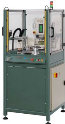
Rotary indexing table with LCN 131
