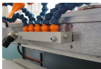
The pad air diffuser device can be mounted with screws laterally .
